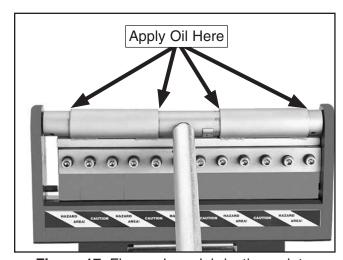
Figure 17. Finger clamp lubrication points.
